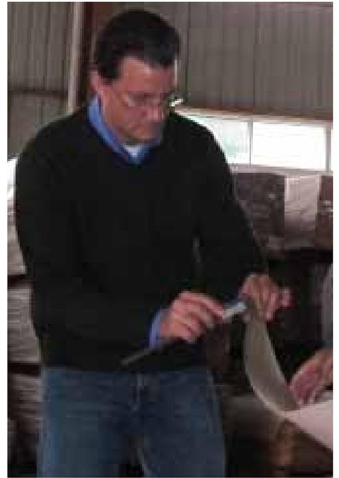
factory group in Anji (Zhejiang province) China [above photo], Vice President of Operations Tom Goodham personally measured thicknesses on all four sides of each sheet of veneer that was destined for Haiku airfoil construction to ensure that our precision manufacturing was going to meet the tight specifications set by Big Ass Fans.
